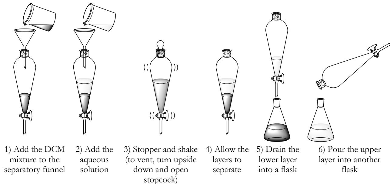
Figure 6-4: Steps in a liquid-liquid extraction performed with a separatory funnel.
