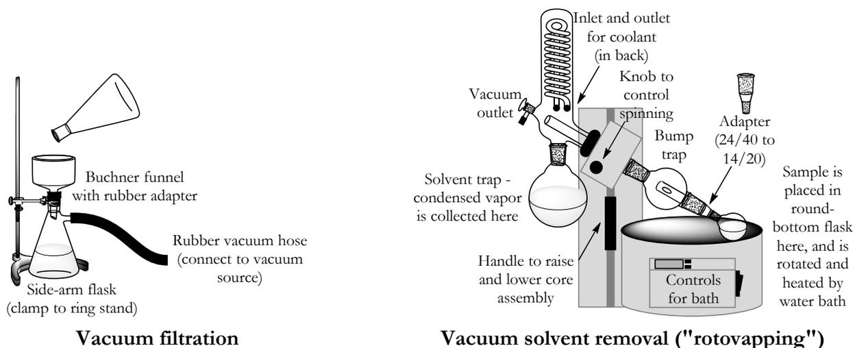
Figure 6-5: The setups for vacuum filtration and vacuum solvent removal.
