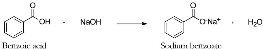
Figure 6-2: Benzoic acid is deprotonated with base.
