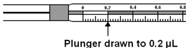
Figure 9-3: Drawing up 2 µL of liquid into the syringe.
