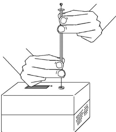
Figure 9-4: The correct method for injecting a sample into a Mini GC.
