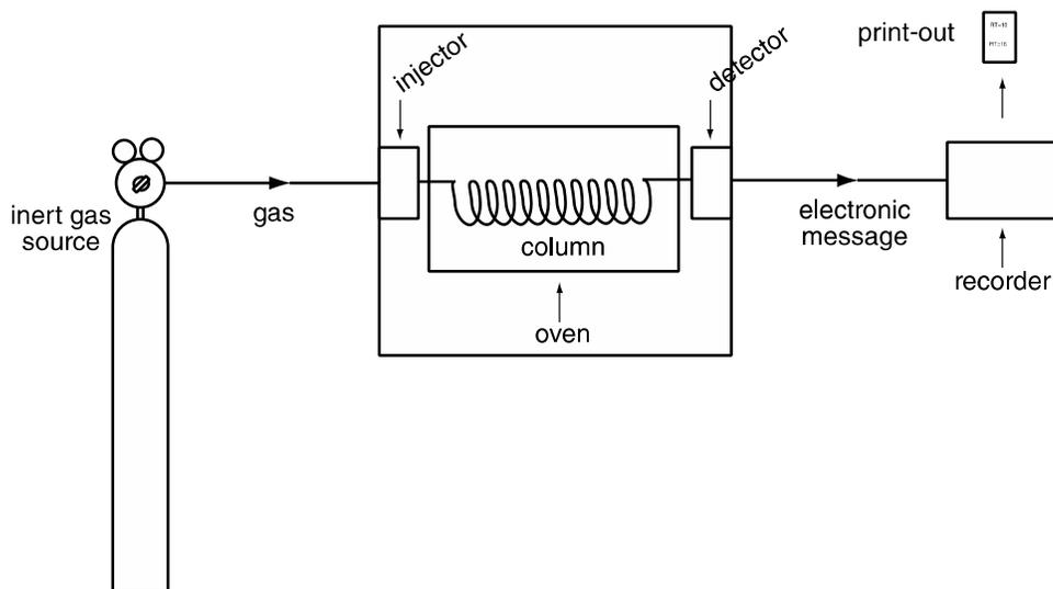
Figure 9-1: Schematic of a gas chromatograph (GC).
