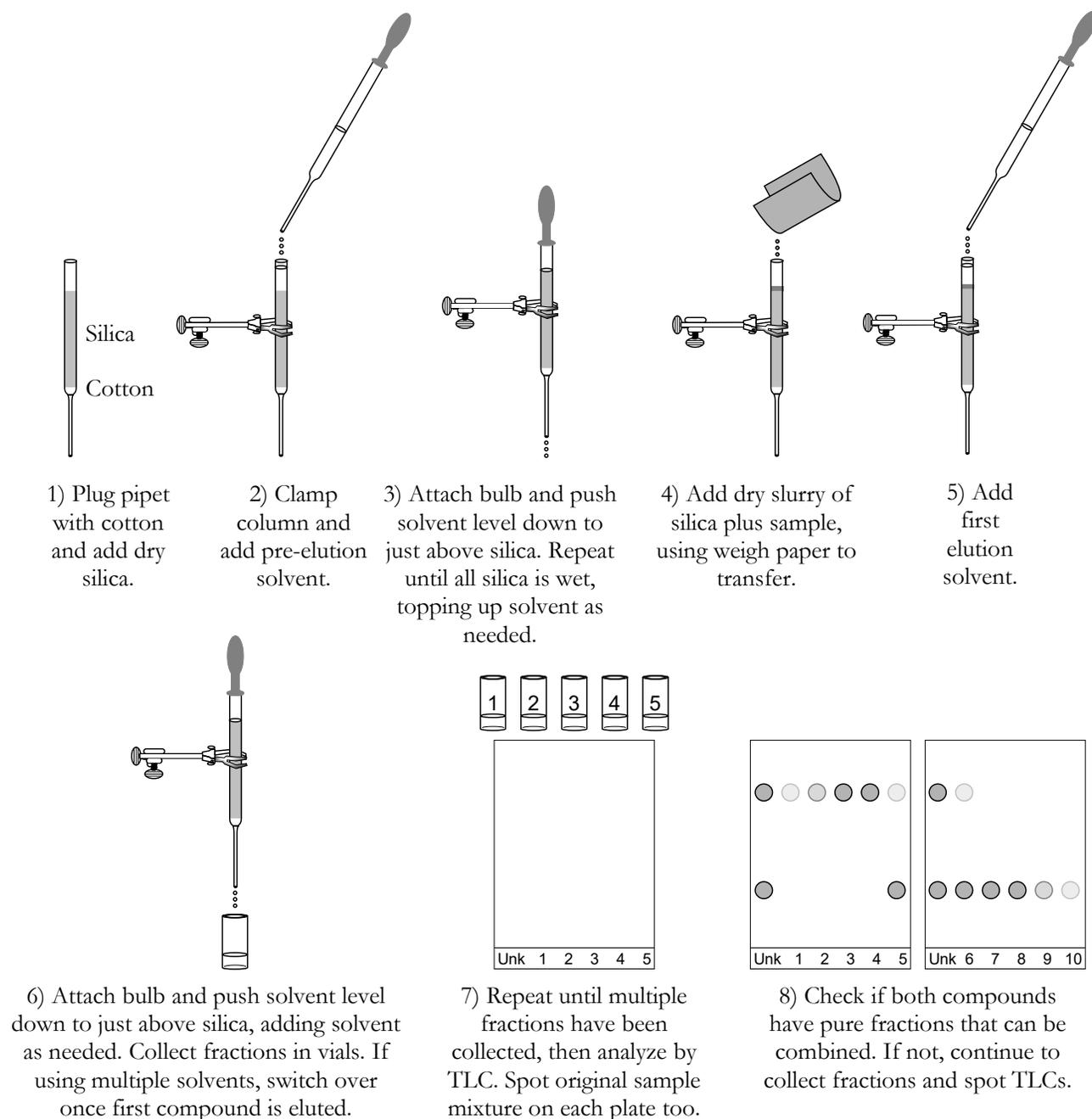
Figure 8-3: The procedure for microscale column chromatography.
