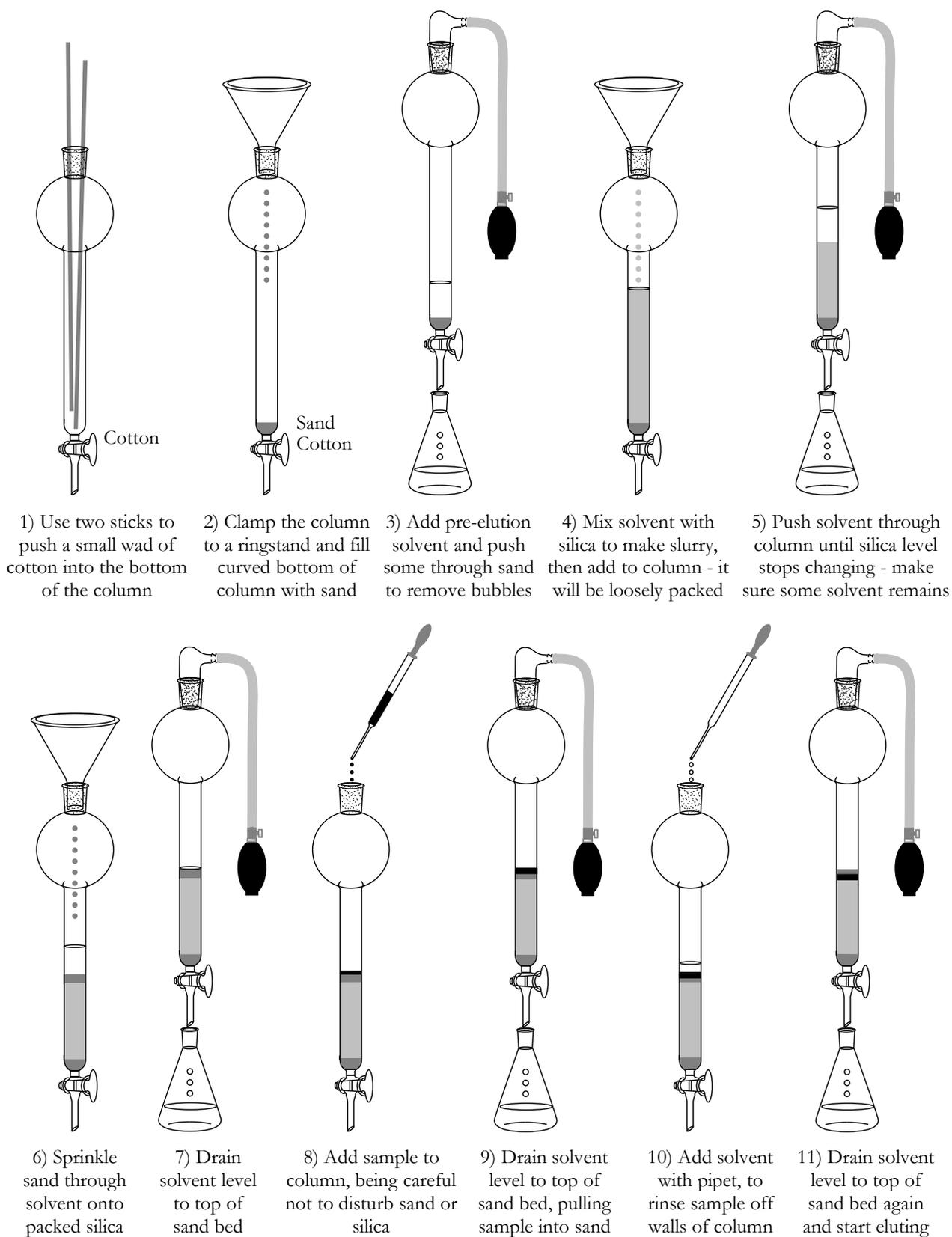
Figure 8-5: Steps for performing column chromatography on a large scale, using solution loading.
