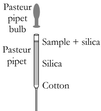
Figure 8-2: A microscale flash column can be performed with a Pasteur pipet.
