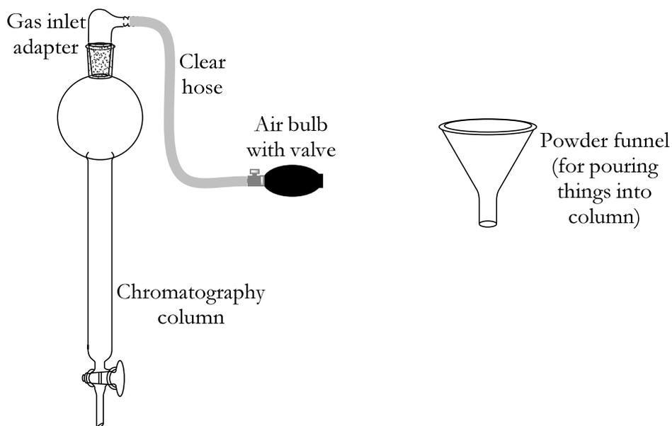
Figure 8-4: Glassware for large-scale column chromatography.
