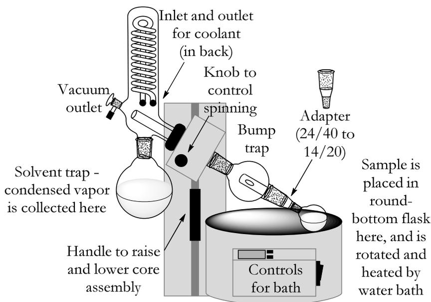
Figure 14-1: The general layout of a rotary evaporator, or rotovap.
