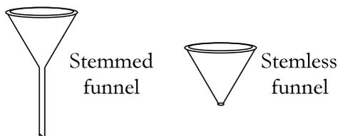
Figure 13-3: Glassware used for gravity filtration.
