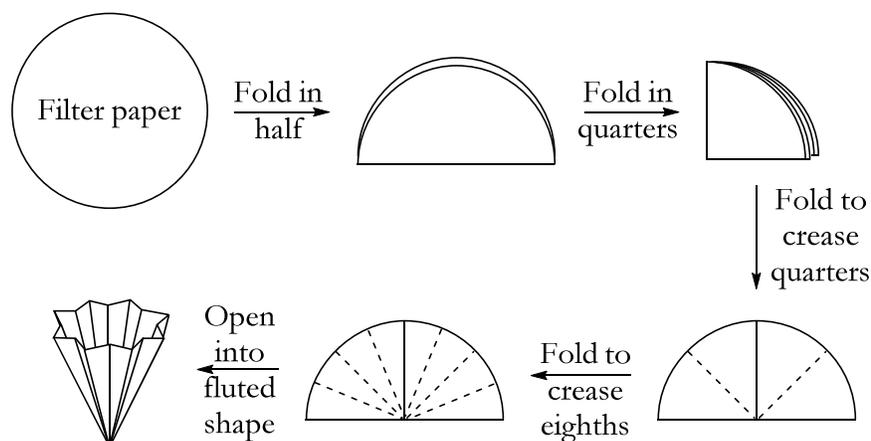
Figure 13-5: The procedure for folding a fluted filter.
