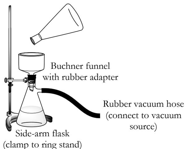
Figure 13-2: Setup for vacuum filtration.
