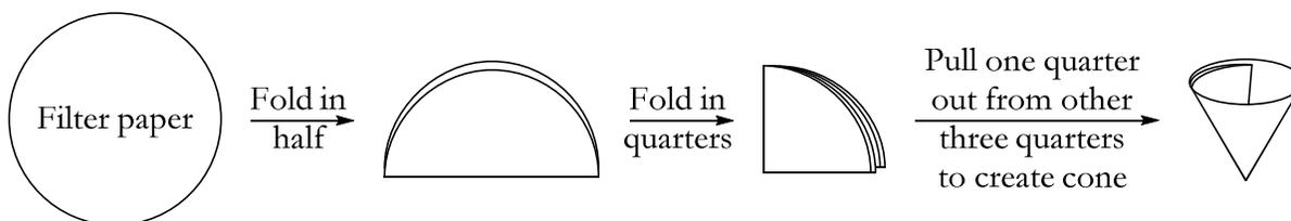
Figure 13-4: The procedure for folding a cone-shaped filter.
