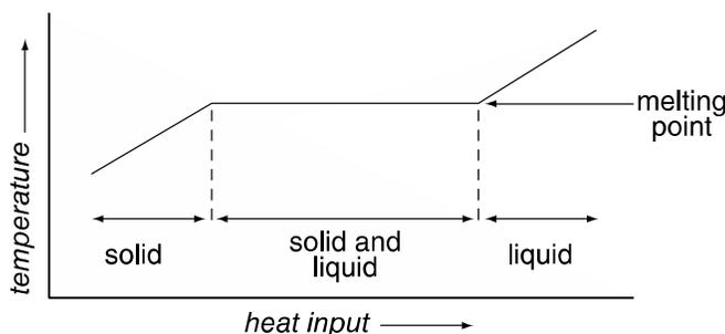
Figure 10-1: Melting behavior of solid compounds.
