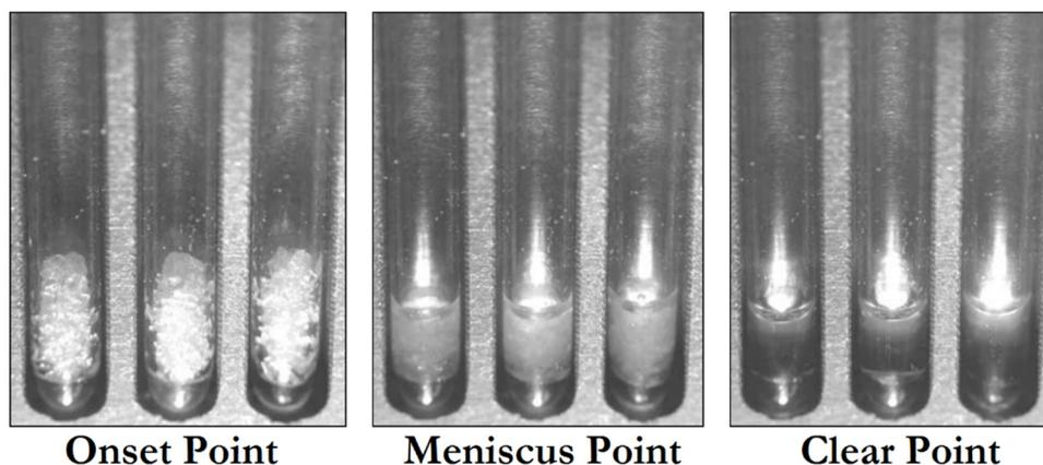
Figure 10-2: The onset point, meniscus point, and clear point are the three most important visual observations.
